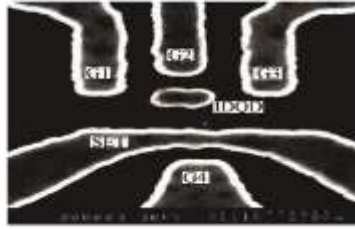
Figure 9.37. Photomicrograph of the structure for a quantum computer in a scanning electron microscope
